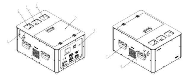
1/8: Side output nozzle hole 2/3/4: Top panel output nozzle hole 5: Fuel tank cover 6: Rear panel 7: Handle
