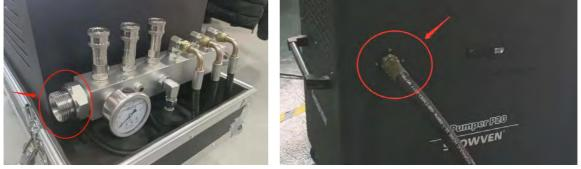
**Branch hose 3/8 DN10 installation:** When installing the branch hose, the end which with Y-shaped filter is installed on the flame head uFlamer X20, and the other end is installed on the accumulator module. Both ends are hydraulic quick coupler.
