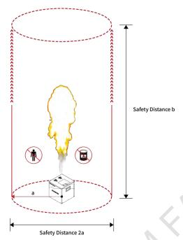
The uFlamer Gasboom safety isolation zone (show as above) is a cylindrical three-dimensional space with safety radius around machine (a) and safety distance at firing direction (b). For safety distance at firing direction equals to maximum firing height+2m. No person and flammable materials are allowed to stay inside the safety isolation zone when flamer was armed. Unauthorized persons and objects are strictly prohibited from entering.
