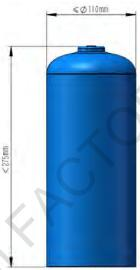
Cartridge holder for 4 support cartridge with outer diameter is less than or equal to  $\phi 66 mm$ , and the height is less than 275mm.
